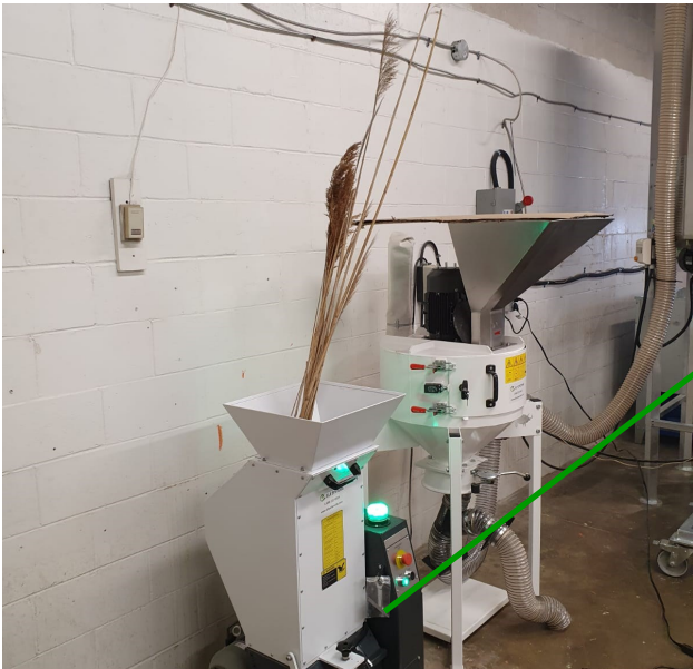
Fiber shredder for wool, bamboo, hemp stalk etc. Staggered carbide blades and easy access for cleaning.
