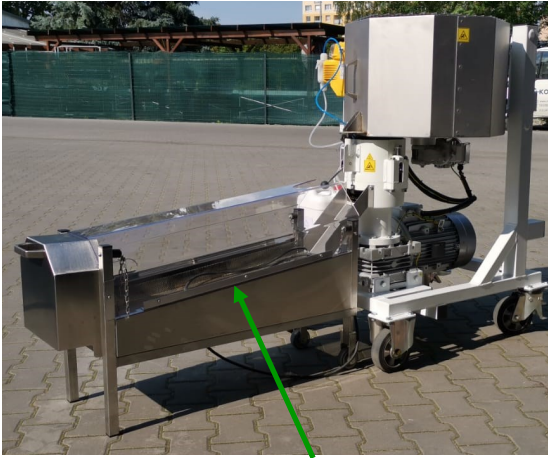
Stainless steel vibrating pellet cleaner with plexiglass hood for operator observation 7.5kw shown removes small fibers and allows the waste to be re-pelleted
