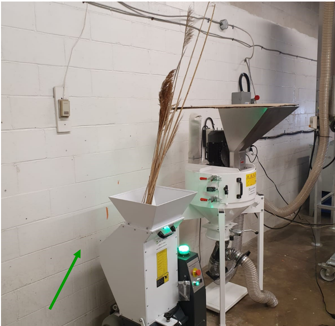
Hammer mills and shredders: Built with carbide blades and heavy duty hammers, dust control built into each unit.
