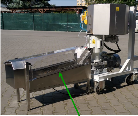
Stainless steel vibrating pellet cleaner with plexiglass hood for operator observation 7.5kw shown
