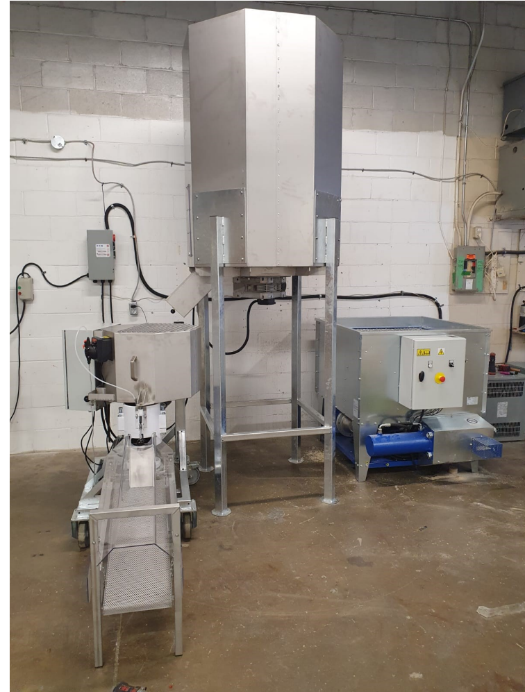
1.2 or 2.5 m3 fully stainless steel hopper, for larger scale grinding and pelleting. The hopper includes a gear driven sweep arm and feed chute for easy dosing of the pellet mill hopper.
